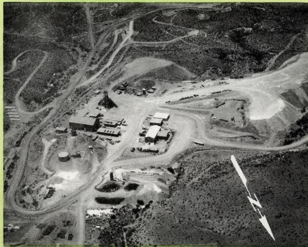
During the present program of mine development all men and materials enter the mine through No. 1 Shaft. The mine dump shown on the right contains over one-third million tons of stockpiled ore.
