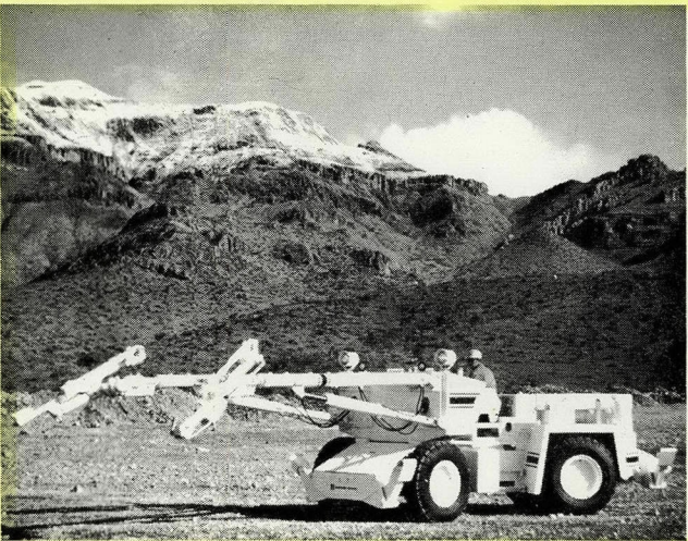
Two boom drill jumbo, one of six used for drilling blast holes in the underground development headings.
