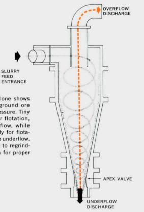
Cross section view of a cyclone shows where the slurry of finely-ground ore and water is fed in under pressure. Tiny particles, properly sized for flotation, are carried off in the overflow, while larger particles not yet ready for flotation drop out by gravity as the underflow. This material will be subject to regrinding and then cycloned again for proper classification.
