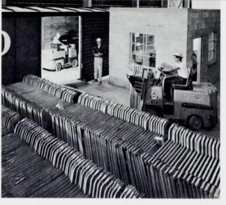
Anodes, after being approved by Quality Control, are picked up, several at a time, by fork-lift trucks and loaded in railroad cars for shipment to the electrolytic refinery.
