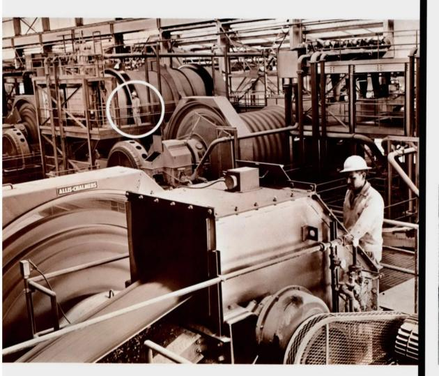
The "wet grinding" cycle begins when the minus-half-inch ore is mixed with water and fed into the six Grinding Sections at Kennecott's Concentrator in Hayden. Each of these sections is headed by a rod mill for coarse grinding, ball mills for fine grinding and cyclones for classification.
