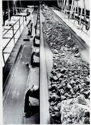
At the bottom of the Track Hopper there are six hydraulically-operated "feeders" that supply ore to three 48-inch wide conveyor belts. They take the ore up an incline for a distance of 535 feet to a point high inside the huge Crushing Plant.
