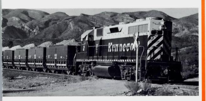
Upon arrival at Hayden, a whole trainload of ore can be unloaded in minutes. The ore cars, of side-dump design, unload their cargo in Kennecott's big underground Track Hopper. Over 50 feet deep, the Hopper has a capacity of 6,000 tons — over  $1\frac{1}{2}$  trainloads of ore.
