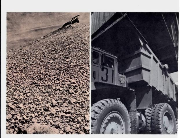
Even a giant haulage truck — upper right corner of photo — looks small compared to mountain of waste rock onto which it is dumping 85-ton load. Material classified as "ore" is hauled by trucks and dumped — one truckload approximately every 5 minutes — into Primary Crusher, which prepares it for shipment to Reduction Plant.
