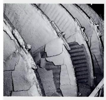
Above: The wet copper "concentrate," which at this stage contains 20% copper, is dried on these disc-type vacuum filters. After being dried, it goes to storage bins — and from there to Smelter Building.
