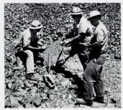
Samples of the rock broken by the blast are taken by Quality Control workmen to be assayed and classified as ore to be milled or material to be leached.
