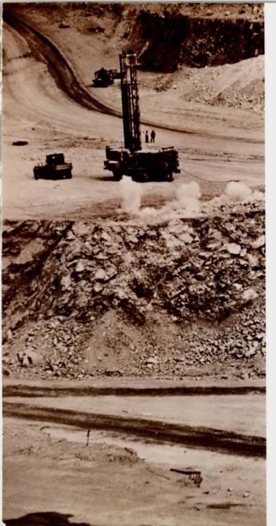
After the blast-holes have been loaded with explosives, the charge is set off (left) and upwards of 40,000 tons of copper-bearing material is broken, ready for loading.
