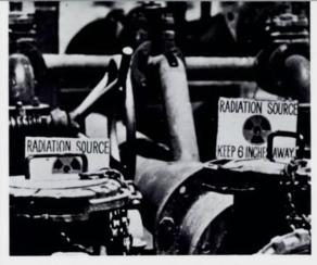
This device utilizes radioactive isotopes to measure density of tailings, and to activate valves which maintain most efficient ratio of water to the waste materials.
