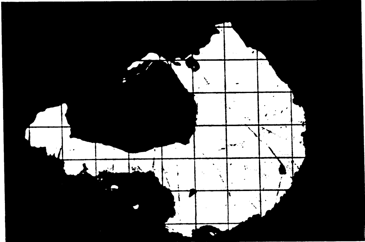
AS&R-1 (H.G.) Polished section photomicrograph of large liberated native gold particle bordered at bottom by minor and poorly polished goethite. Plain light, X435. Each square of grid is 32 microns on an edge.
