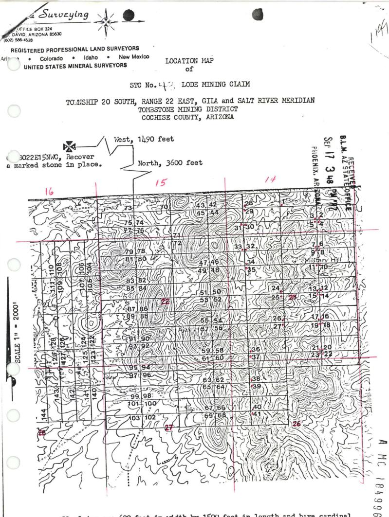
All claims are 600 feet in width by 1500 feet in length and have cardinal bearings unless specifically noted otherwise. All corners and location monuments are marked by wooden posts not less than  $3^n \times 3^n$  by  $4^n$  in height or by white PVC posts not less than  $1^n_{11}$  in diameter by  $4^n$  in height.
