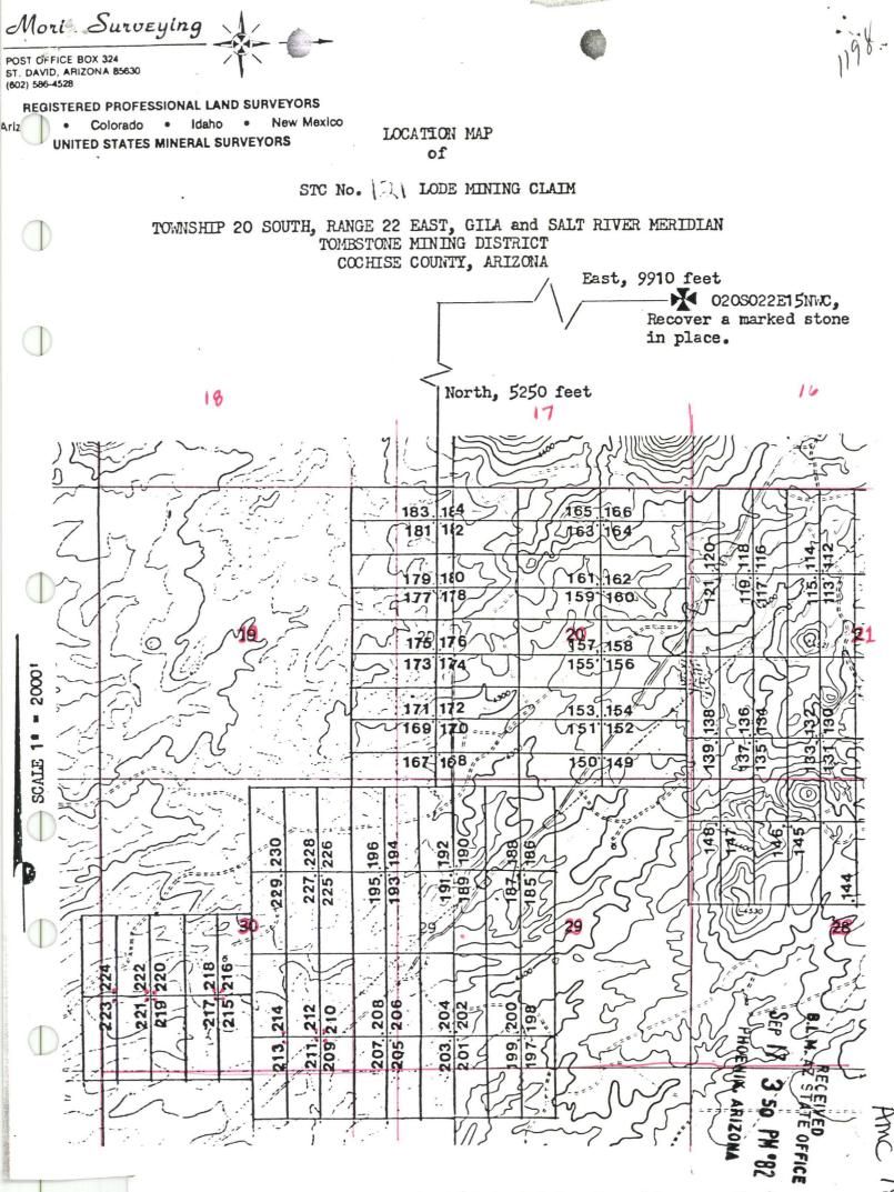
l claims are 600 feet in width by 1500 feet inlength and have cardinal arings unless specifically noted otherwise. All corners and location muments are marked by wooden posts not less than  $3^n \times 3^n$  by  $4^i$  in height by white PVC posts not less than  $1^{2^n}$  in diameter by  $4^i$  in height.
