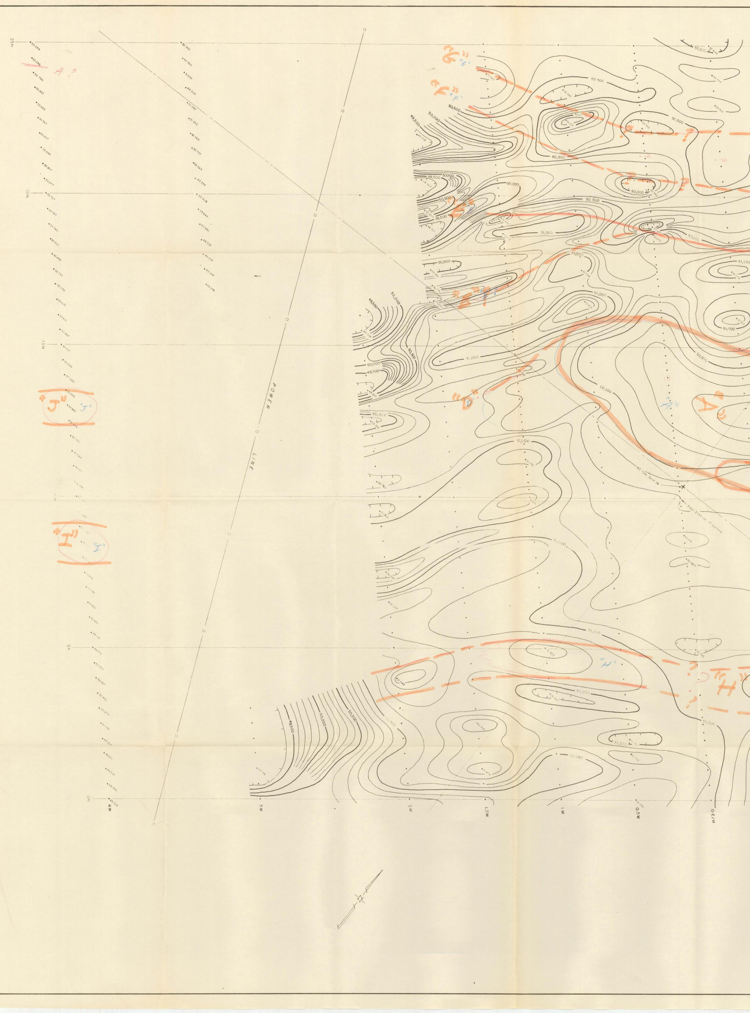
50,500 • 5, . · 54 26 8 . . • . • • \* • • . . • 50 530 0.5 E Ē - • --·50839 2E 1.56 . ° | CONTOUR INTERVAL: 100 GAMMAS TOTAL MAGNETIC INTENSITY CONTOURS of New River Area Maricopa County, Arizona for NORANDA EXPLORATION INCORPORATED by HEINRICHS GEOEXPLORATION COMPANY P.O. BOX 5964, TUCSON, AZ. 85703 JOB NUMBER 1198 AUGUST 1975 . -
