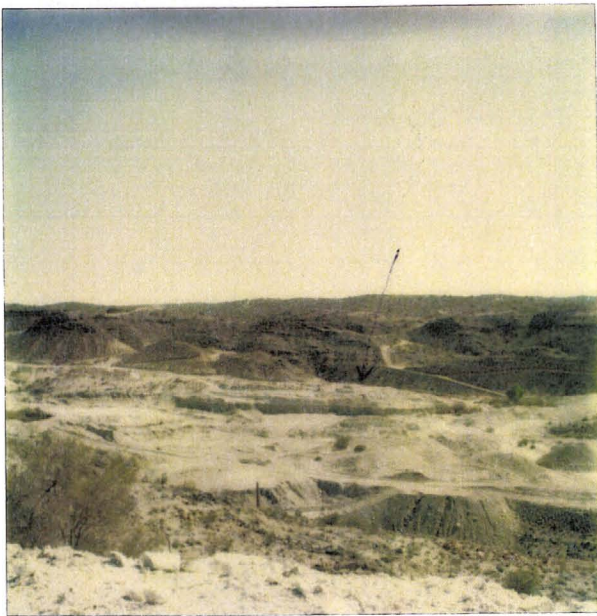
Main pit area of Anderson mine. Arrow points to other photo. Photo looking south (down dip). The pit bottoms in main mineralized zone. White beds are silic. ls. Dark beds (ridge formers) are upper conglomerate and ls.
