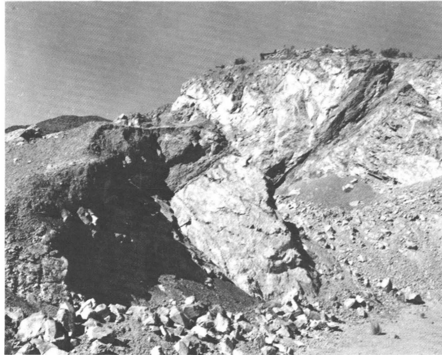
Photo 17. The Emsco silica quarry operated by Gladding McBean and predecessors from 1928 to about 1945. The light-colored quartzite of map unit 7 is cut by a darker sill of granitic rock. The quartzite was used in manufacture of silica brick. Photo taken in March 1960, observer facing northeast.
