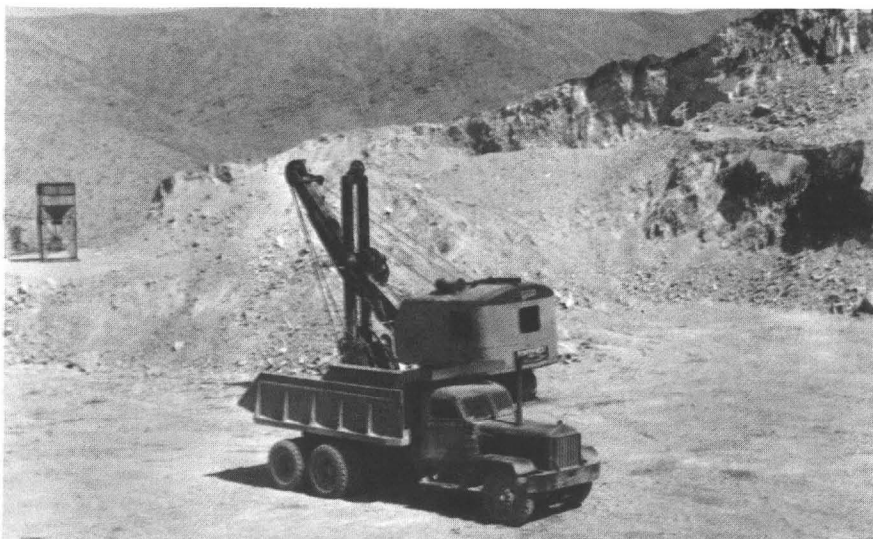
Photo 16. The Atlas quartzite quarry of Mineral Materials Company as seen in 1956, observer facing southeast. The company has produced 150,000–200,000 tons of quartzite since 1939, mostly for use by portland cement plants.
