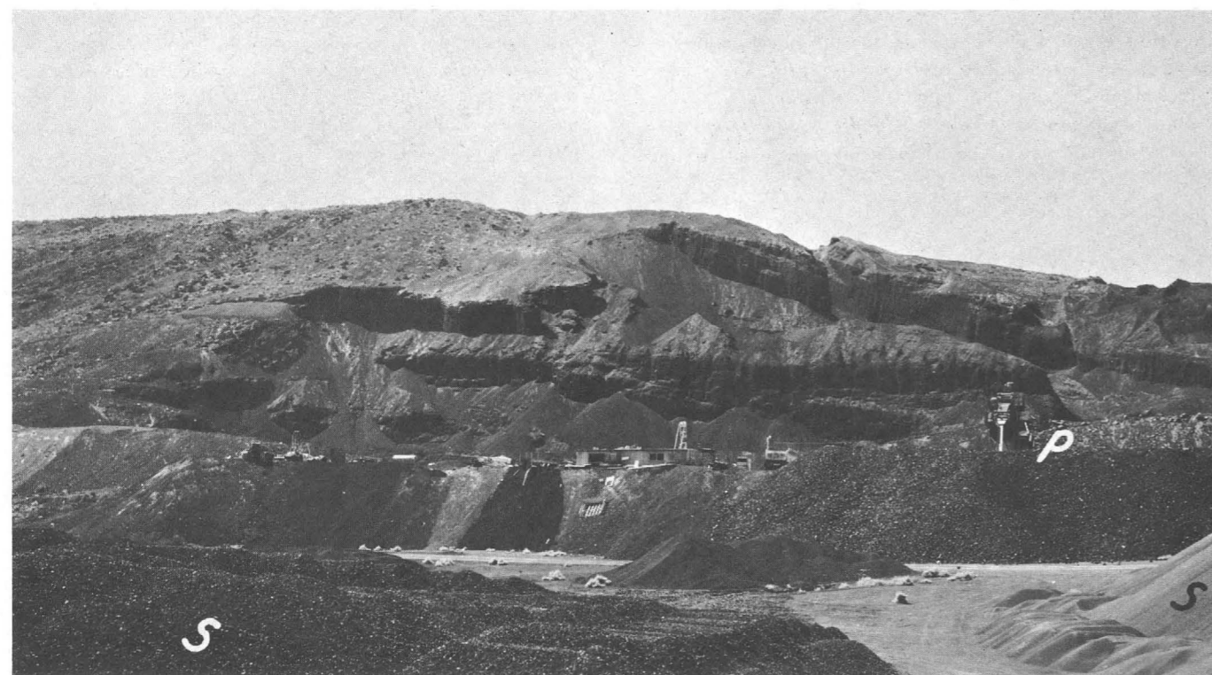
Mining cinders at Cima Cinder deposit. Cinders are well bedded and contain volcanic bombs. The processing plant is in the right center (P), and the stockpiles (S) are below. View is west.
