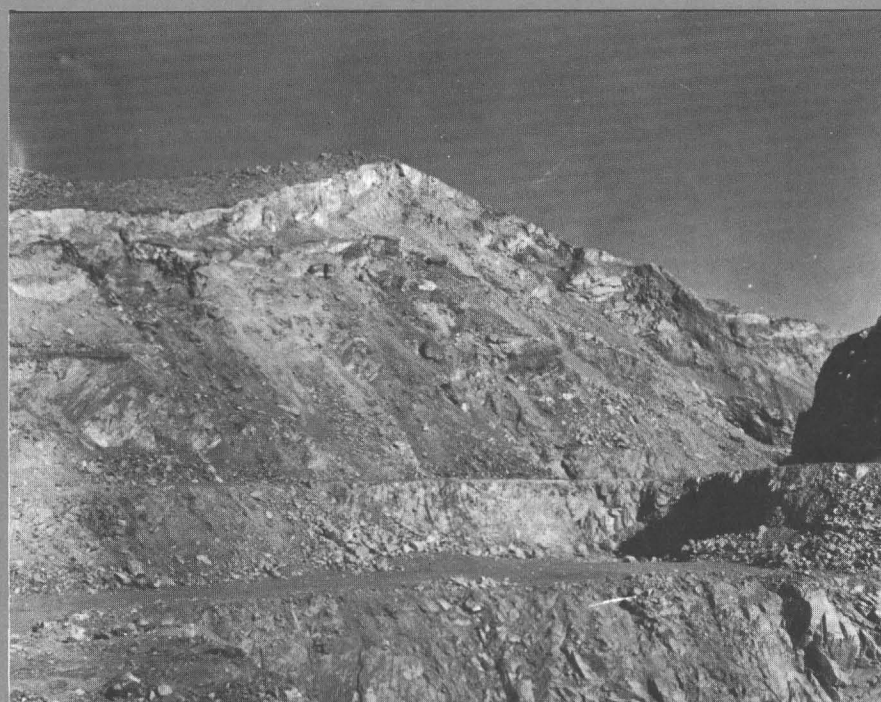
Photo 6 (left). Klondike limestone quarry of the Riverside Cement Division of the American Cement Corporation near Oro Grande, in March 1960 (observer facing southeast). The mass of broken slide rock, which is chiefly limestone, is being removed to supply part of the cement plant requirements. It is gradually sliding down one of the surfaces of the Klondike fault. Quartzite of map unit 7 occupies the left skyline.
