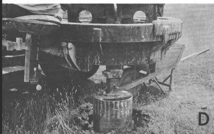
(A) Division of Mines geologist (F.R. Kelley) marking selected drilling site by stake. (B) Rig is moved into position. (C) Close up of drill bucket showing bits used for drilling. Extra bits are lying on top of the collar. (D) Spudding in. (E) Drilling contractor (L.W. Ecker) operating drill. (F) Sample emptied from drill bucket by driller's helper (Richard Robles). (G) Hole nearing completion. Samples are laid in rows, each representing 20 ft. of hole. (H) Division of Mines geologist examining sample.
