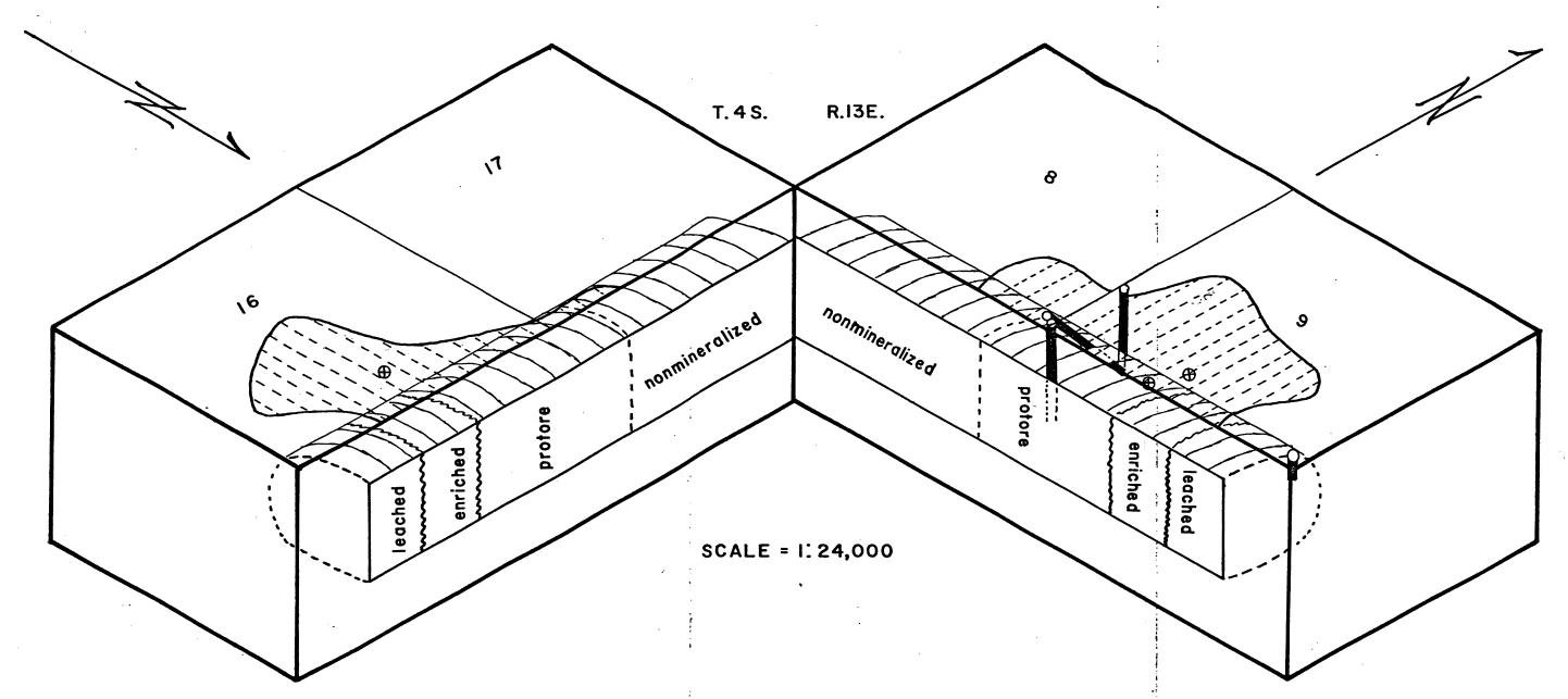
ISOMETRIC DIAGRAM SHOWING HYPOTHESIZED TARGET AT THE KELVIN PROSPECT - A CYLINDRICAL BODY OF LARAMIDE AGE QUARTZ MONZONITE HAS BEEN ROTATED TO THE EAST 60°-90° SINCE EMPLACEMENT AND IS PRESENTLY SURROUNDED BY THE ORACLE GRANITE OF PRECAMBRIAN AGE. INDUCED POLARIZATION ANOMALY ON THE SURFACE (red) INDICATES UNDERLYING SULFIDE ZONE. PAST DEEP DRILLING HAS BEEN TOO FAR WEST TO TEST THE MOST FAVORABLE PORTION OF THE TARGET. PROPOSED C.S.M.C. DRILLING SITES =  $\oplus$ .
