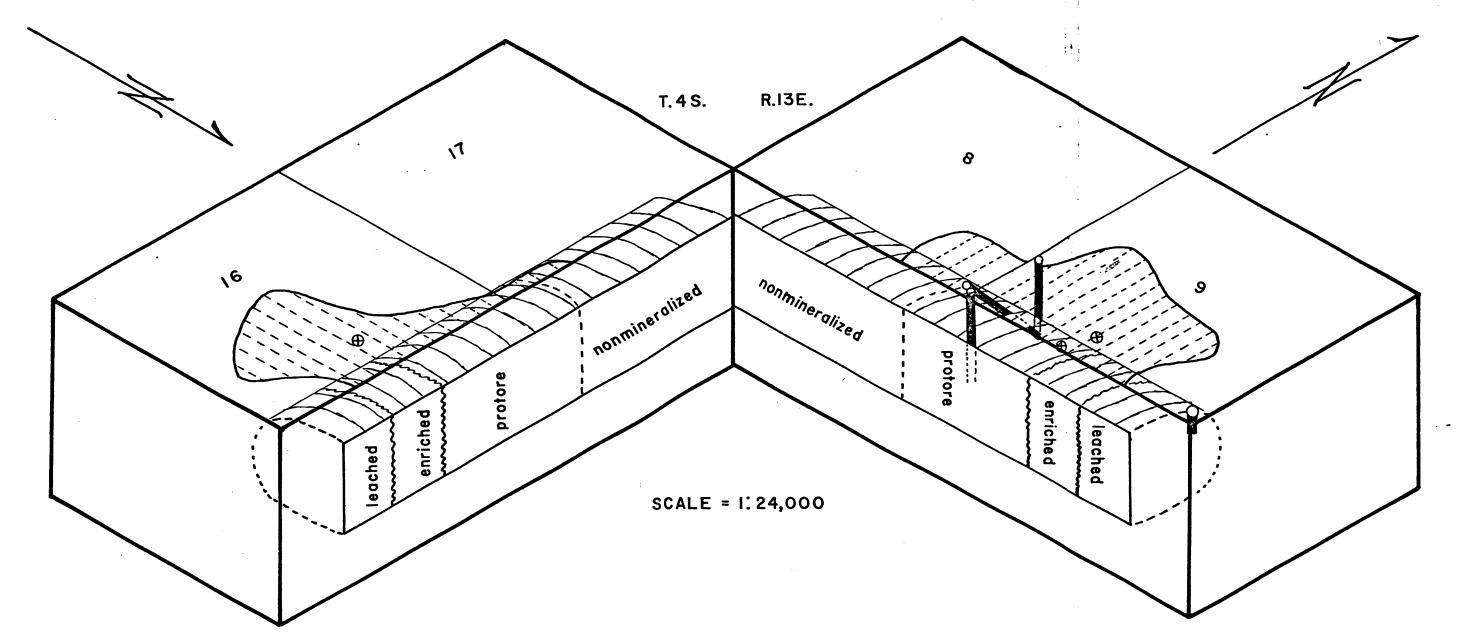
ISOMETRIC DIAGRAM SHOWING HYPOTHESIZED TARGET AT THE KELVIN PROSPECT - A CYLINDRICAL BODY OF LARAMIDE AGE QUARTZ MONZONITE HAS BEEN ROTATED TO THE EAST 60°-90° SINCE EMPLACEMENT AND IS PRESENTLY SURROUNDED BY THE ORACLE GRANITE OF PRECAMBRIAN AGE. INDUCED POLARIZATION ANOMALY ON THE SURFACE (red) INDICATES UNDERLYING SULFIDE ZONE. PAST DEEP DRILLING HAS BEEN TOO FAR WEST TO TEST THE MOST FAVORABLE PORTION OF THE TARGET. PROPOSED C.S.M.C. DRILLING SITES =  $\oplus$ .
