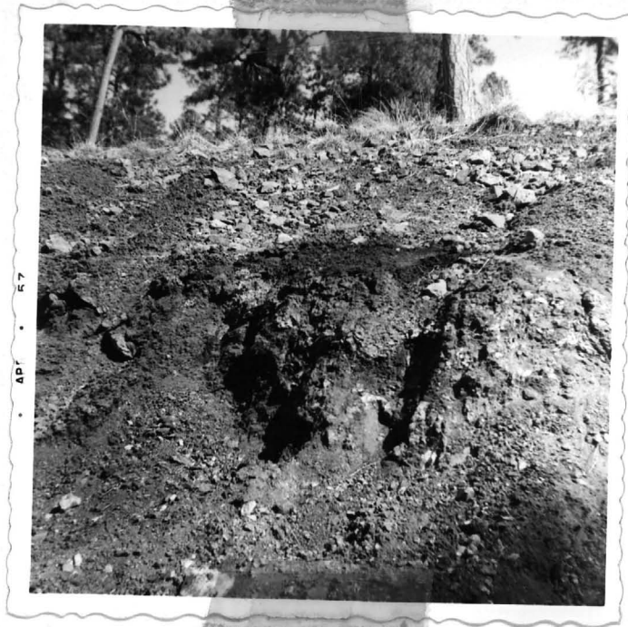
Photo 3 -Looking north into face of open cut just south of owners cabin on Rainbow No. 12 claim. Shows heavy concentration of manganese mineralization in clay and sandy loam.
