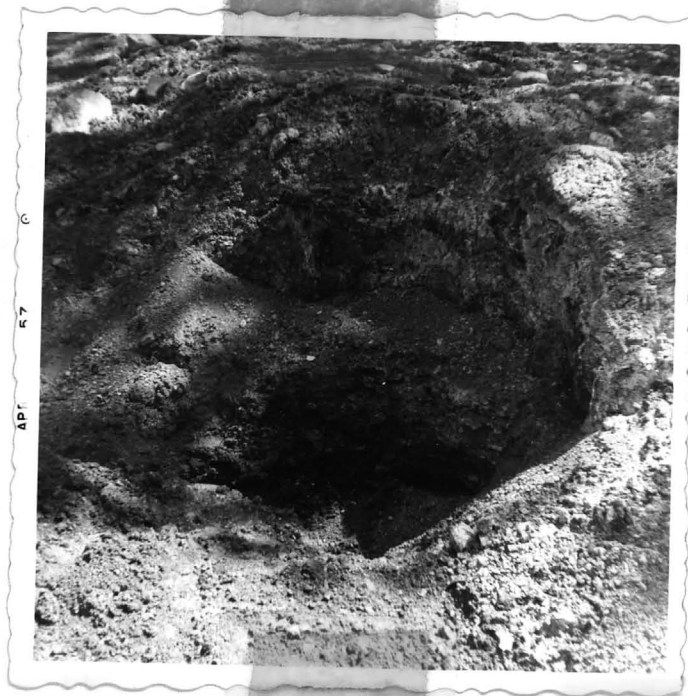
Photo 4 -Shows lenses and heavy concentrations of manganese mineralization in pit on Royal Blue No. 2 claim. Looking south.
