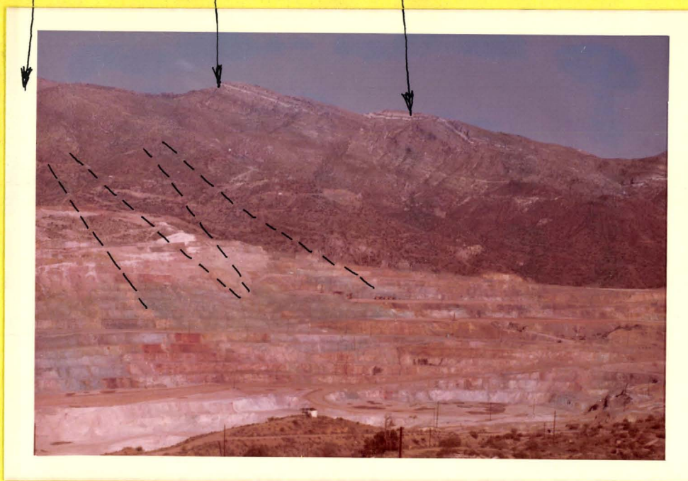
Photograph taken from Public observation Area of Kennecotts Pearl Handle Open Pit (copper) on the West Bank of the Pit. Looking East to East Bank of Pit and Dripping Springs Mountains in the background. Note sediments in mountain range, displacement of sediments by faulting and possible antioclinal limb resulting from intrusive action to north, or left of picture.
