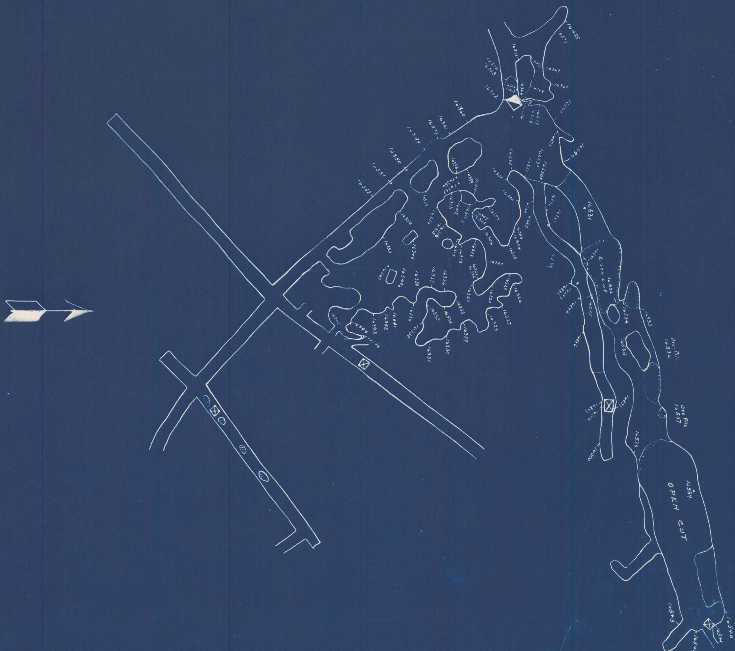
ASSAY - MAP OF PART OF NORTH-WEST STOPES OF TOUGHNUT MINE BETWEEN 1 ST LEVEL & SURFACE SCALE: 1" = 25'
