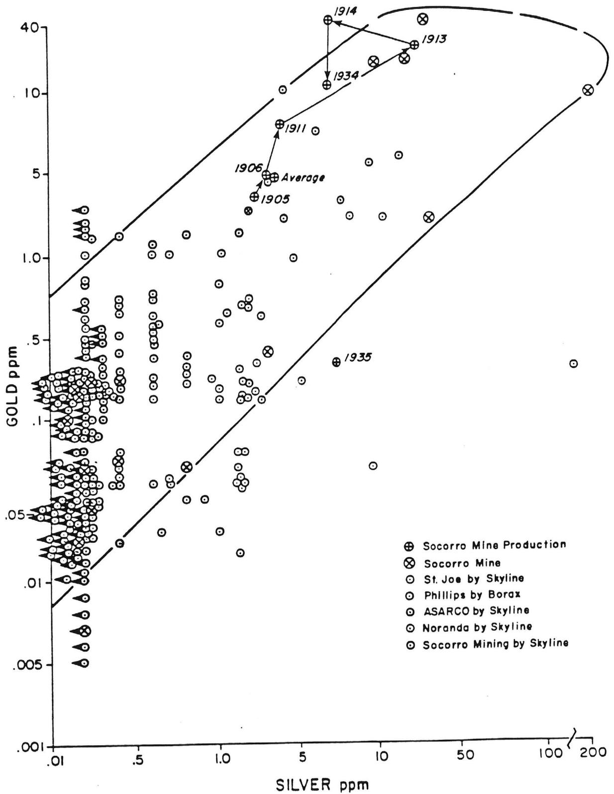
Figure 30. Gold:Silver variation diagram for samples within the Socorro Reef Gold anomaly.
