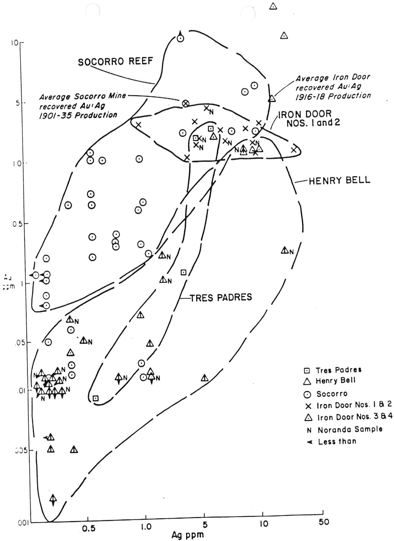
Figure 9. Gold:Silver variation diagram for geochemical samples from mines within the Socorro Peak area of the Harquahala district.
