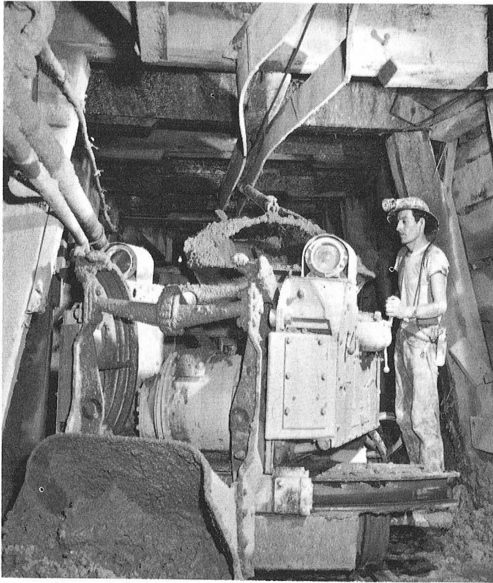
FIGURE 59. - Track Cleaner Modified to Take Power From Trolley Line.
