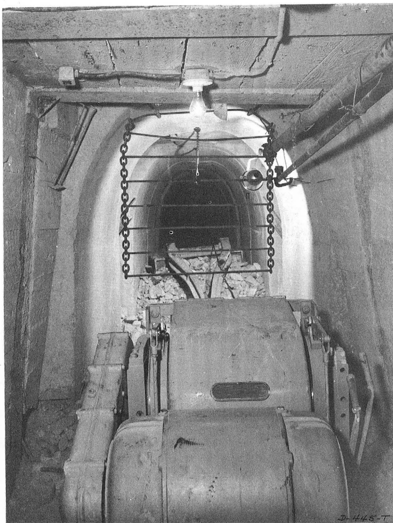
FIGURE 30. - Double-Drum Hoist and Scraper in Concrete-Lined Slusher Grizzly Drift.
