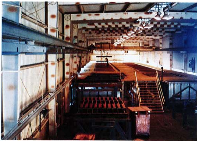
Copper cathodes are grown in an electrowinning facility.
