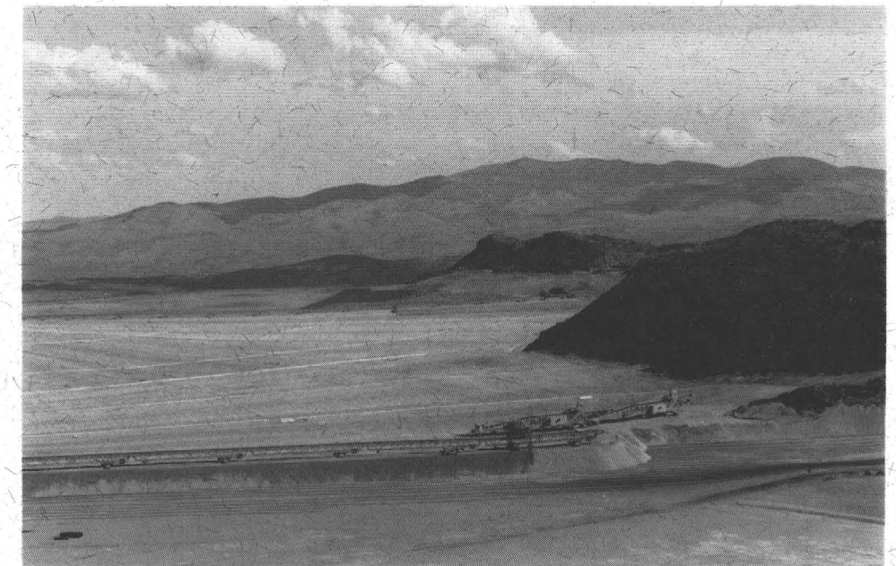
Two 2,000 feet long radial arm stackers construct 22.5 foot lifts and then advance on new material at the high grade Stargo Canyon leach field.
