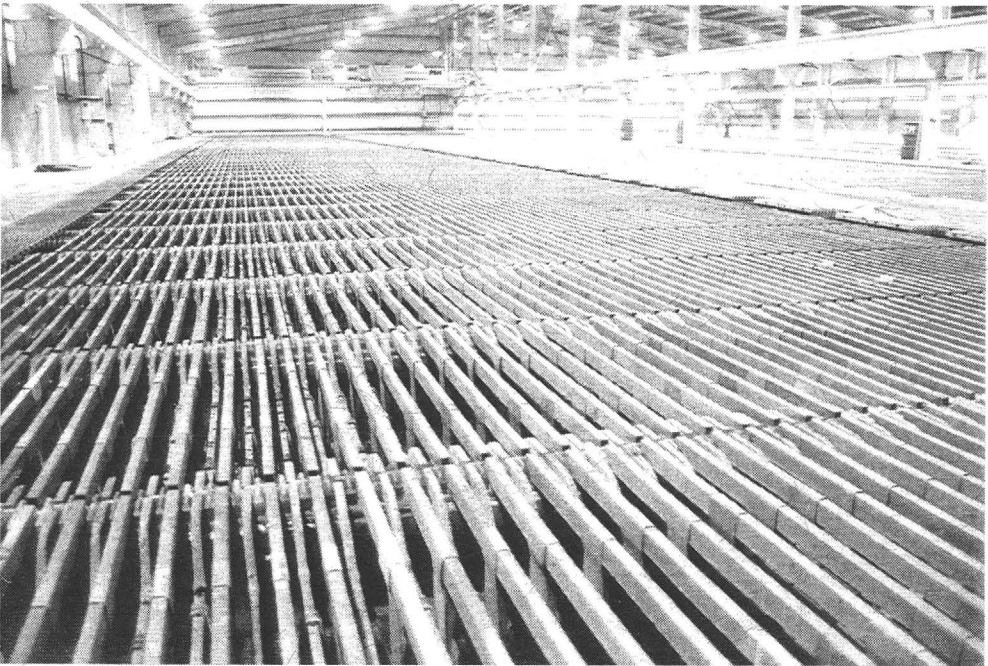
Phelps Dodge's Morenci Hydrometallurgical Division is utilizing a Process Information Management System (PIMS) to streamline processes and optimize flow rates. Dynamic information can be shown in a variety of graphic formats. The electrowinning tankhouse is shown at left.
