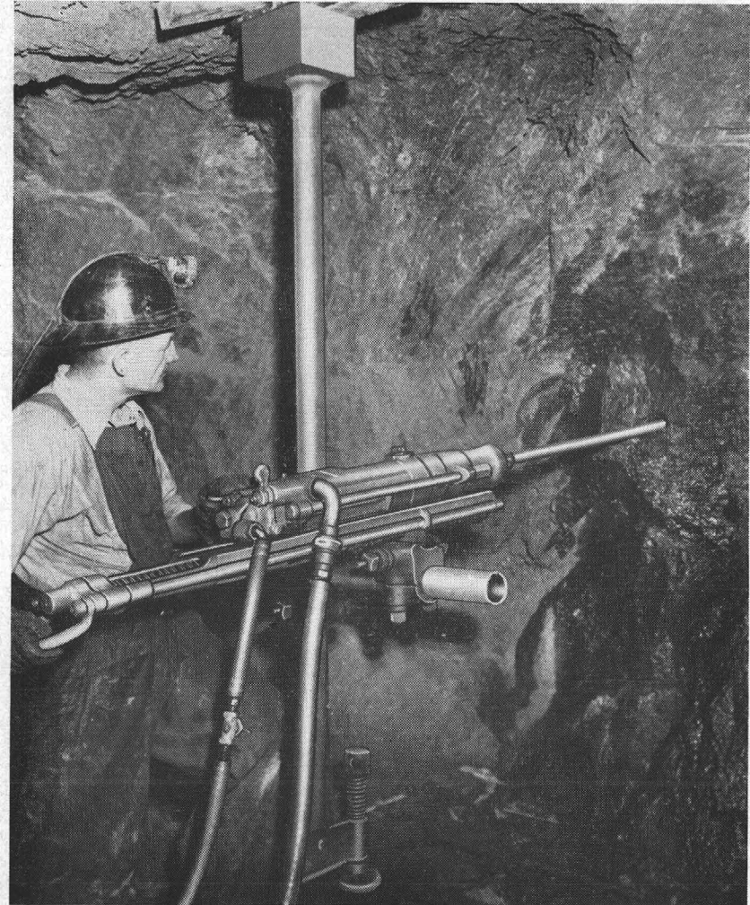
Drilling Blast Holes (Courtesy Chicago Pneumatic Tool Co.)
