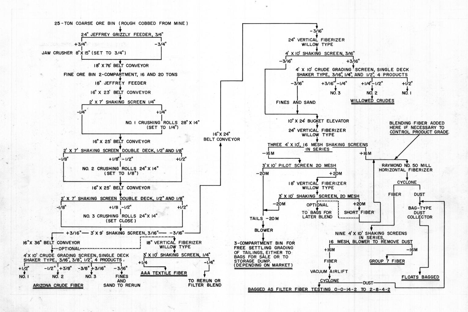
Figure 35. Flowsheet of highway 70 mill, Jaquays mining corporation.
