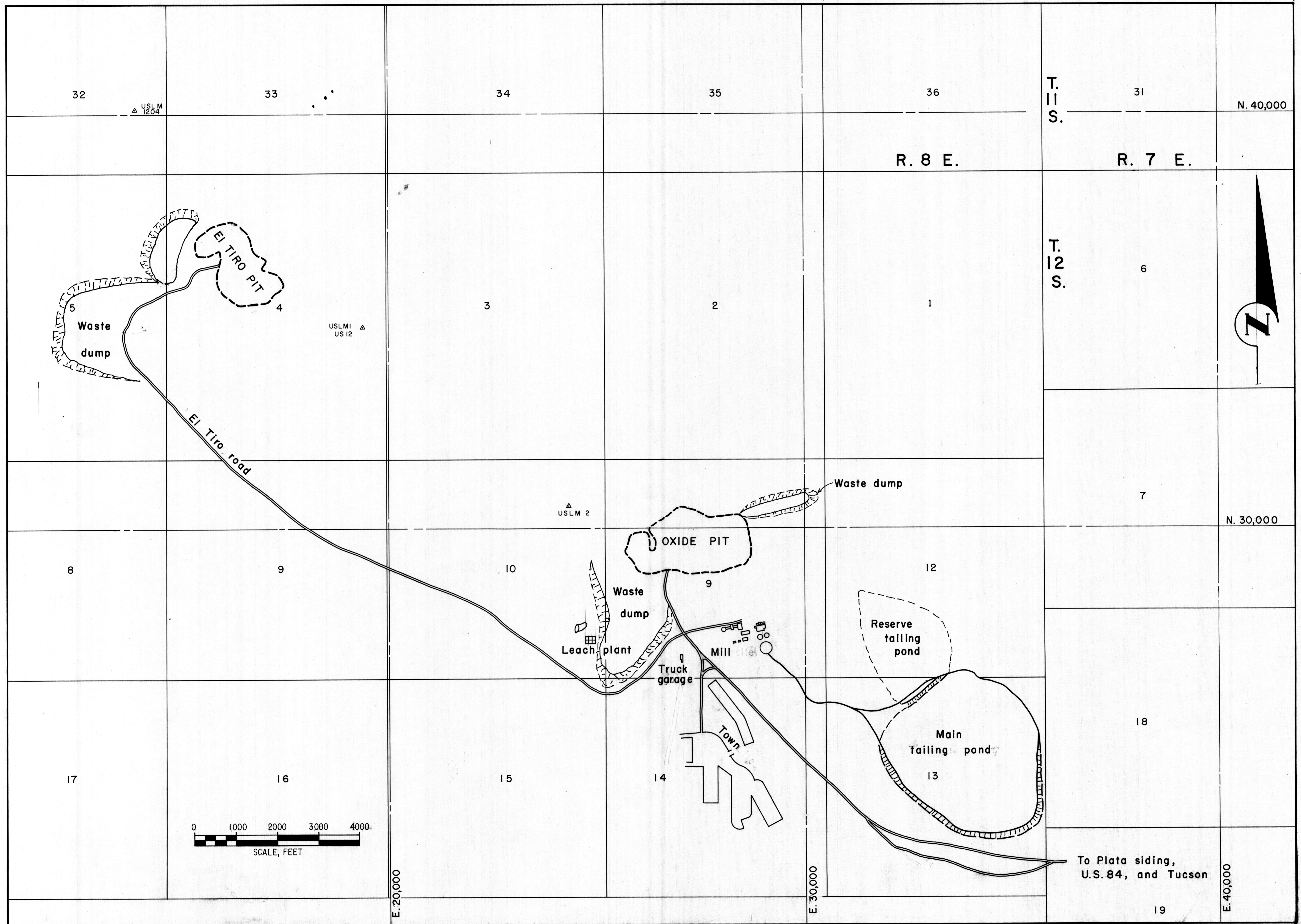
Figure 9.- General Arrangement of Mine Plant
