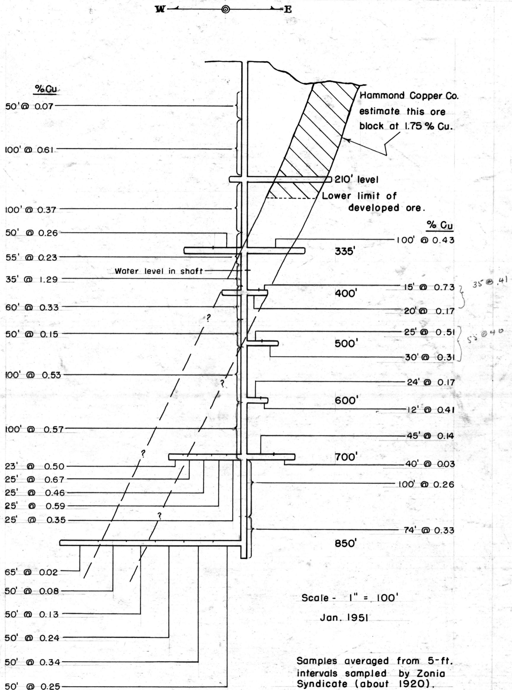
Figure 2. - Cross section, McMahan shaft, showing assays.
