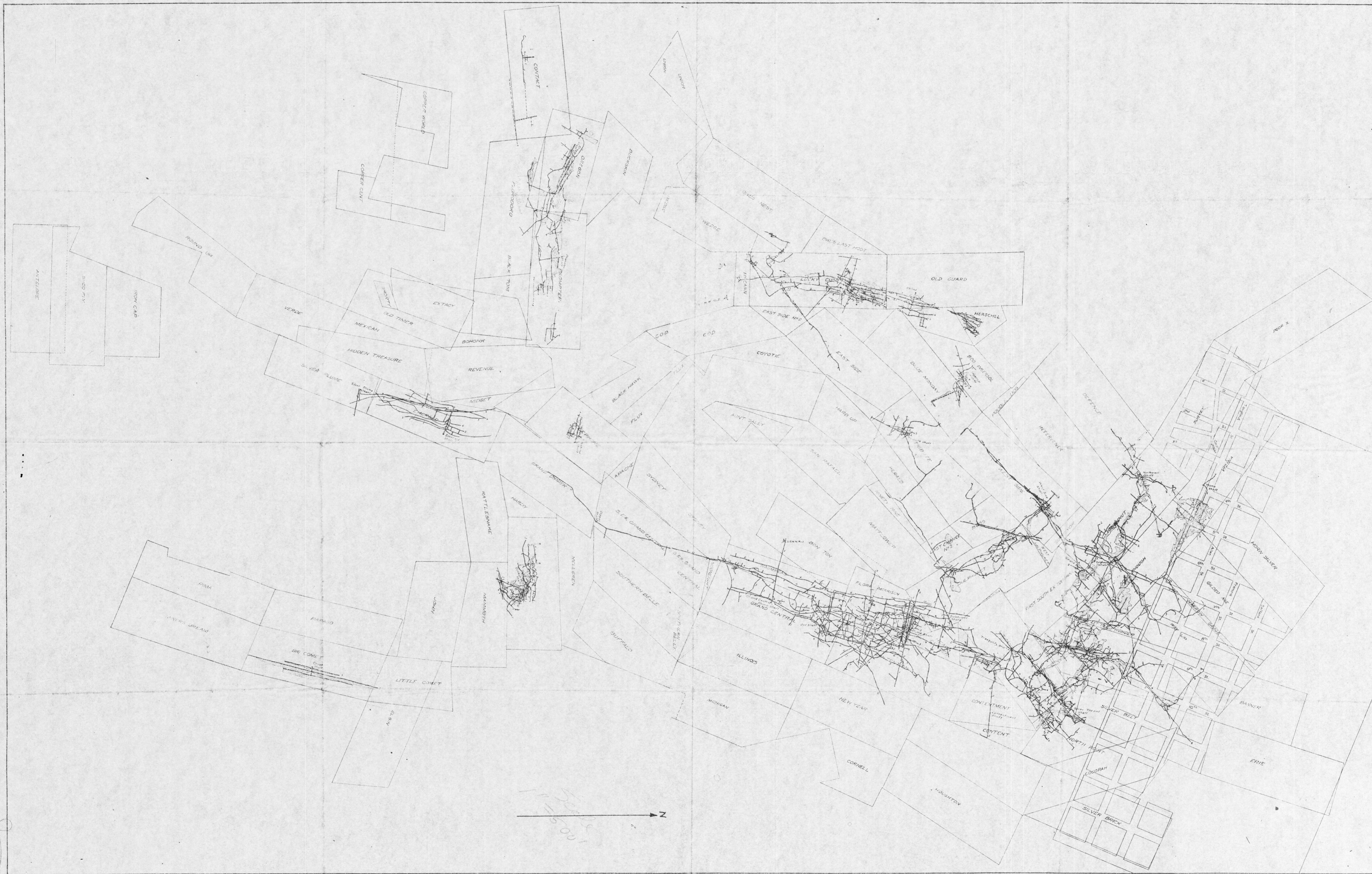
Plate VII.—Map of principal claims and workings in central part of Tombstone district (place transparent paper over Plate IV). Mine levels are indicated by numerals and stoped areas by dots.
