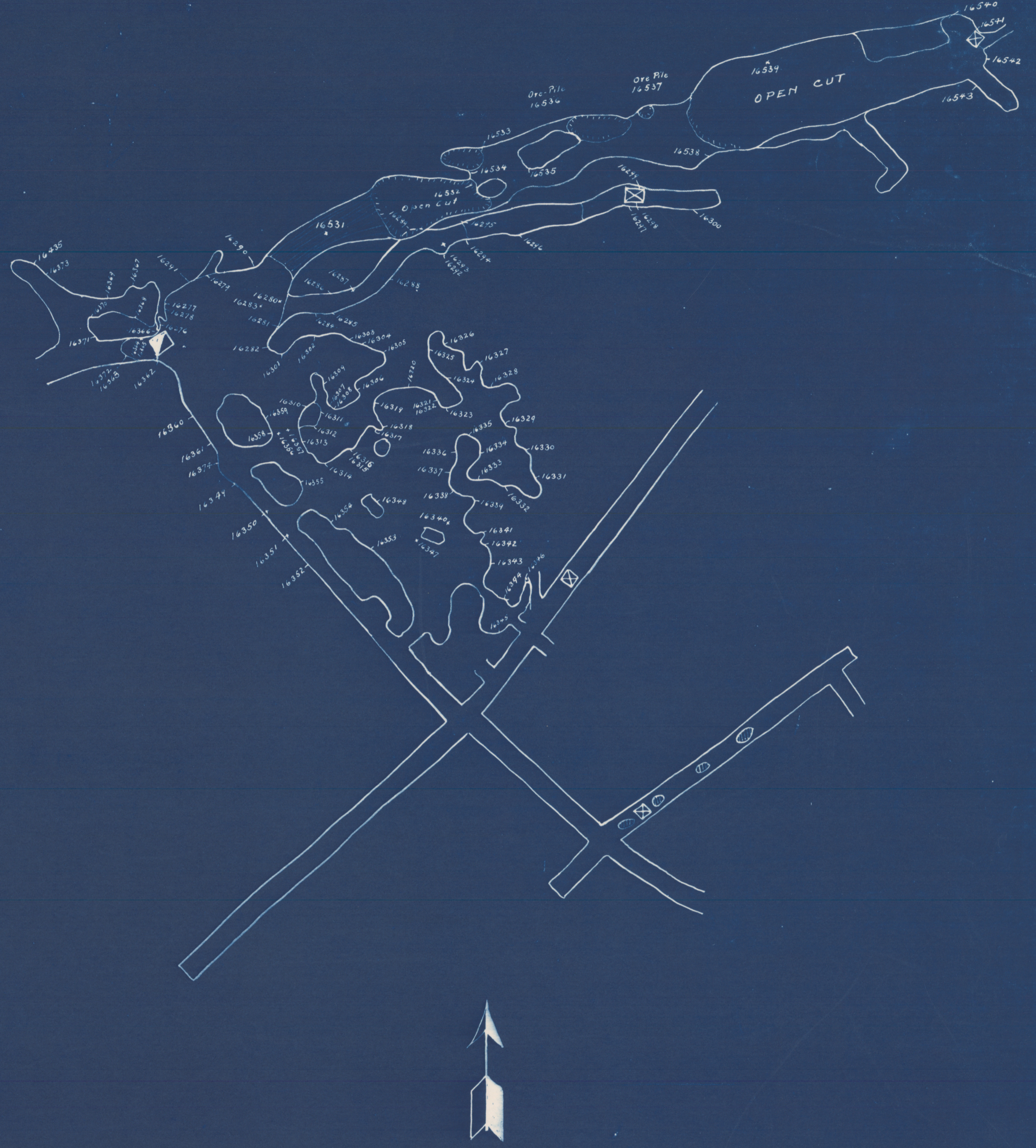
ASSAY - MAP OF PART OF NORTH-WEST STOPES OF TOUGHNUT MINE BETWEEN 1 ST LEVEL & SURFACE SCALE: 1" = 25'
