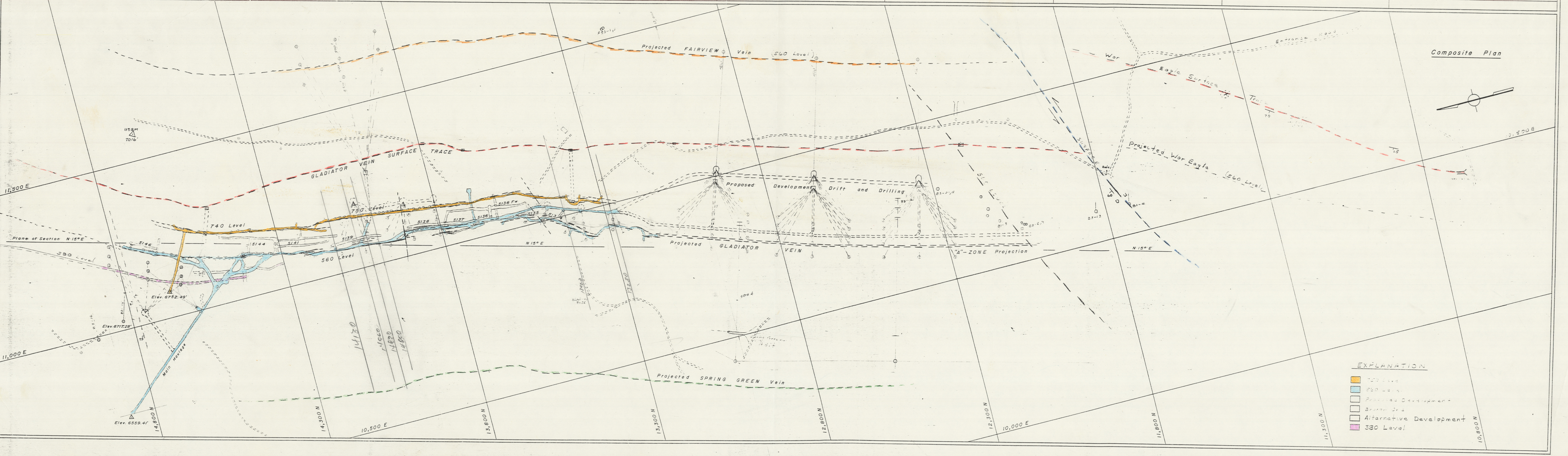
GLADIATOR - WAR EAGLE VEIN Vertical Longitudinal Section Plane of Section N15° E (Looking East) SCALE: 1:1200 0 50' 100' 200' 300' 400' 3-12-88 J.P.P.
