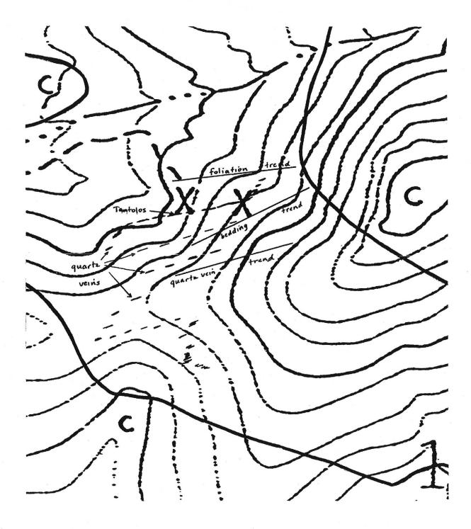
Figure 3: Sketch of relationships between foliation, deformed stratigraphy and quartz veins in the Tantolos Mine area at 1" = 250 feet. Geology by Phillip Anderson, 1989.
