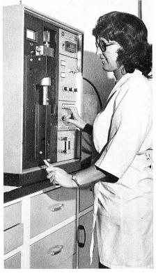
Another invaluable tool of Quality Control is the Oxygen Analyzer at the MP. It is important to know the oxygen content of Silicate Ore Leach Plant cathodes and here's Spectroscopist Sandy Wade making such a determination. Shavings from cathodes are pelletized in sample preparation and these pellets are placed in this machine one at a time for individual assays.
