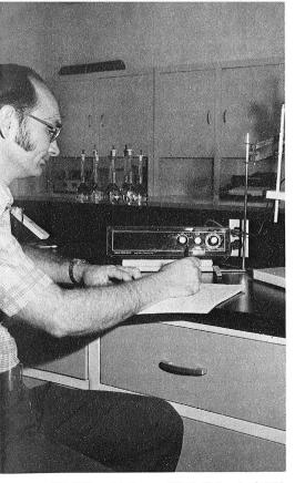
Chief Chemist George W. Self, head of QC's Analytical Services unit, uses the division's pH and Millivolt Meter to check a water sample from some point around the mining operation. This unit with digital readout capability is used primarily to test water samples gathered from points outside the property by the Environmental Control technicians.
