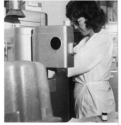
A steady stream of samples of used lubricating oil from division trucks, cars, crushers and mobile equipment pours into the Analytical Services Laboratory for examination and determination of the presence of wear metals. Spectroscopist Sandy Wade does these tests and often these determinations will provide a clue to problem areas which can be corrected before a major engine failure occurs.
