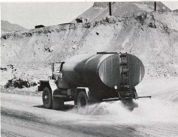
To provide better working conditions for Kennecott's workmen — and to minimize abrasive wear on equipment — dust is controlled by frequently sprinkling truck haulage roads with a chemical-water mixture.
