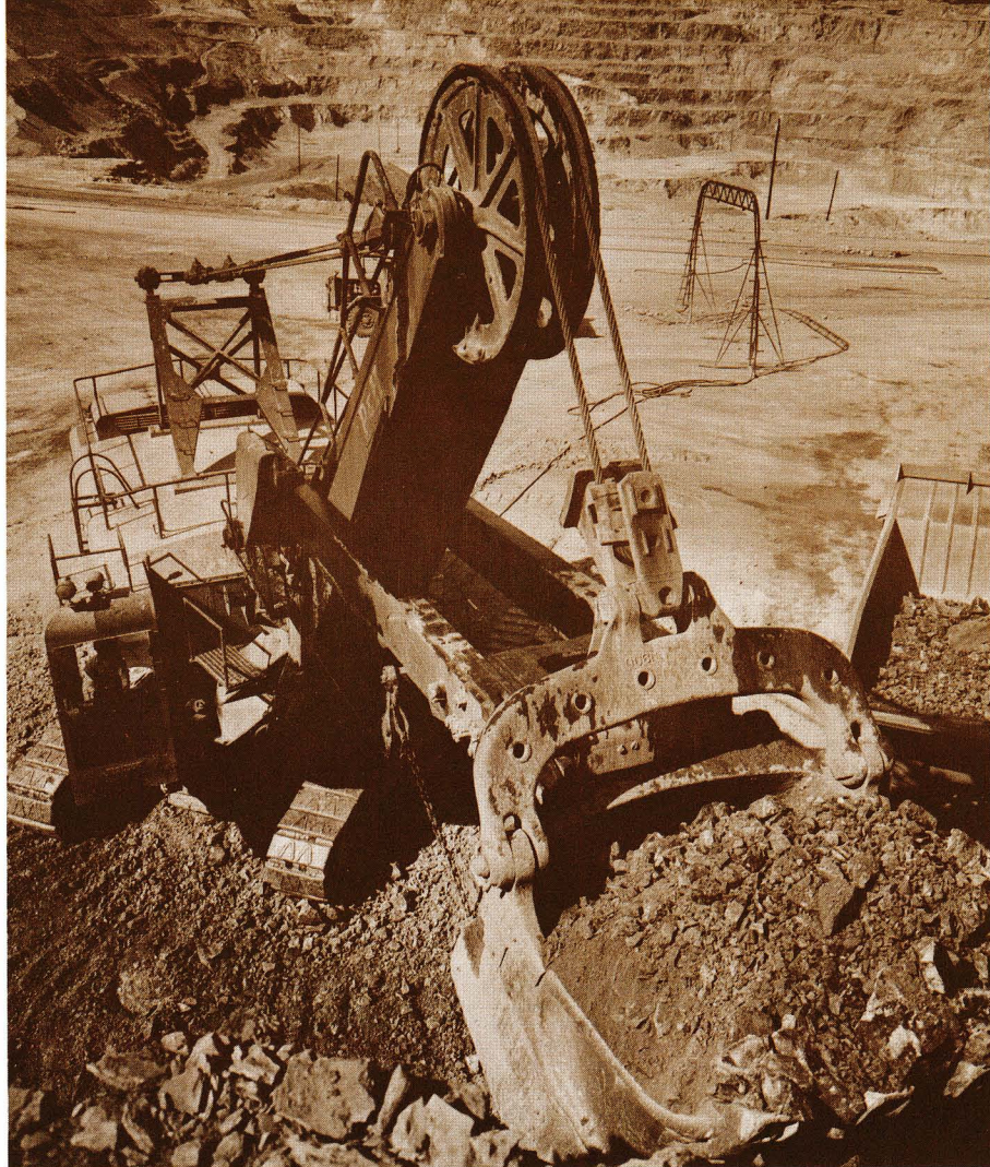
Scooping up 11 tons of blast-broken material at a single "bite," huge electric-powered shovels work night and day loading a fleet of haulage trucks.
