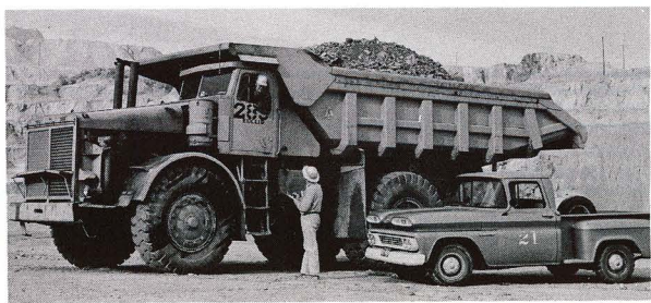
Diesel-powered haulage trucks have 55-ton capacity and two engines, which develop a total of more than 600 horsepower. The truck driver has to climb up to cab on ladder.
