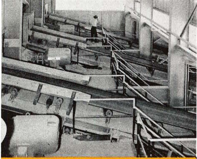
Above: Three conveyors feed ore into the cone-crushers.
