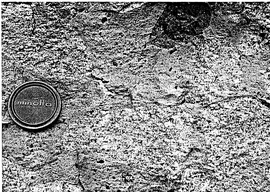
Fig. 4. Detail features of olivine zone, North Pit. Olivine blocks are "salt and pepper" granular masses; the basalt is dark and partially vesicular. Lens cap is 2.5 inches in diameter.
