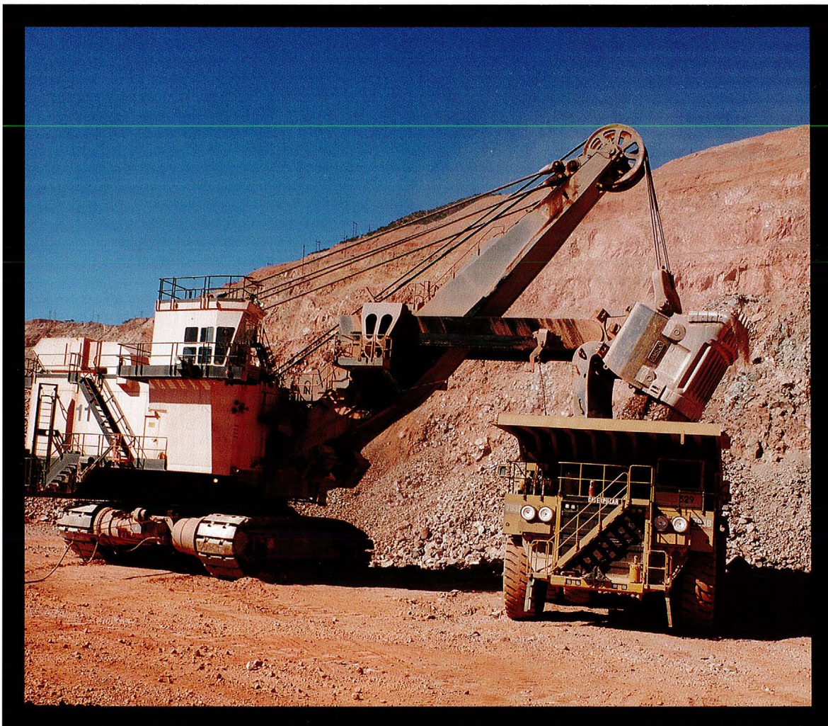
A shovel with 56-cubic-yard capacity loads a Morenci haul truck having a payload of 240 tons.
