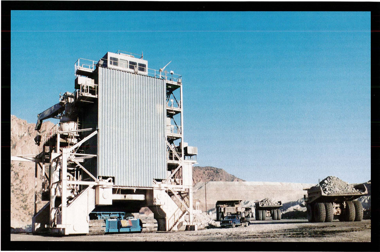
A crawler such as is used to move a space shuttle to its launching pad is shown moving one of the two in-pit crushers to its new operating site within the mine.
