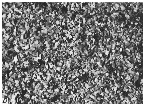
FIGURE 5. - Comparison of hammer mill products and jaw crusher products. A , The concentrate from the hammer mill circuit includes only a few pieces of gangue materials. B , The tailings from this same circuit include only a few pieces of Mica. C , The concentrate from the jaw crusher circuit has many pieces of gangue minerals; they are mostly flat particles. D , The tailings from the jaw crusher circuit contain many pieces of book mica.
