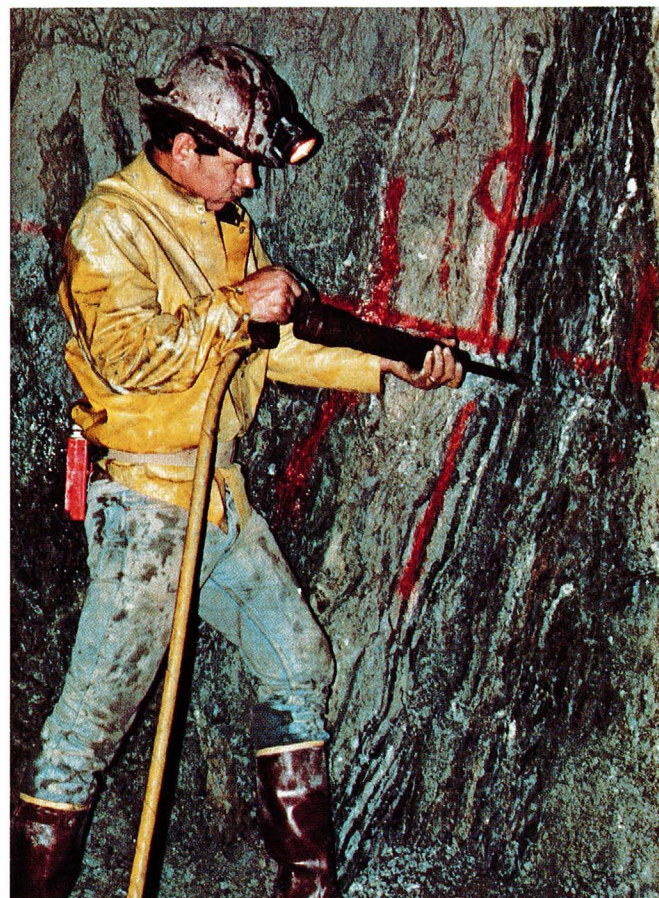
Richard Pape, mine geologist, is shown cutting a channel sample from the north face (N 664.8) on the 1050' level of the McCabe Mine.
