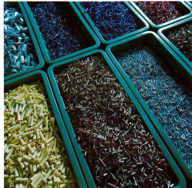
Terminals used to make electrical connections for consumer and industrial products are produced in huge volume at Chicago plant.
