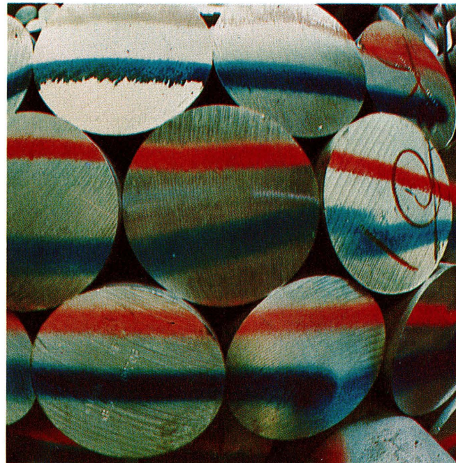
Color-coded aluminum billets identify alloy composition.
