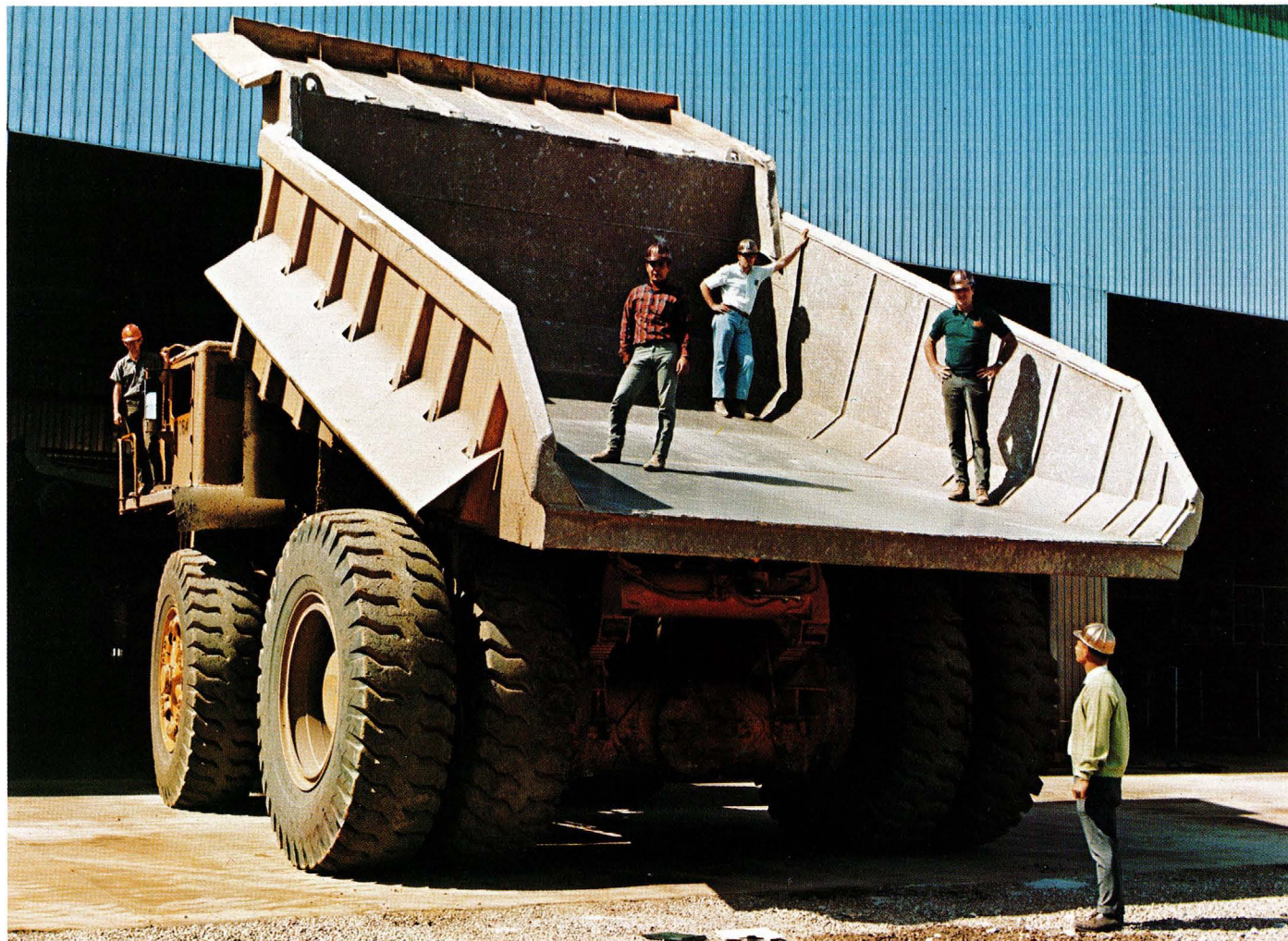
Giant haul trucks used to transport the ore from the benches to the crusher have a rated capacity of 120 and 150 tons. They weigh approximately 110-140 tons empty. Fuel tanks hold 450 to 500 gallons of diesel oil and the 48-ply tires stand nine to ten feet high and weigh some 3000 pounds.
