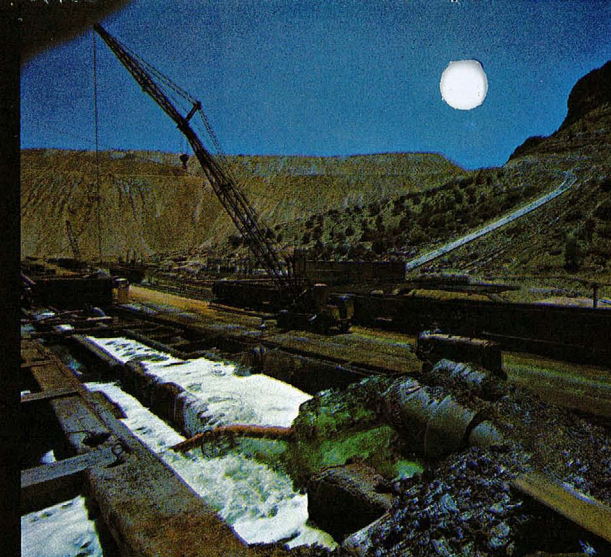
Chino's precipitation and piping to leach areas.
