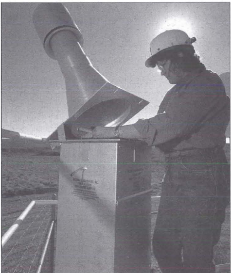
Environmental Scientist Angelee Johnson replaces a filter at an air monitoring site near Black Mesa Mine. The company operates 10 air monitoring stations which provide more than 600 samples annually.
