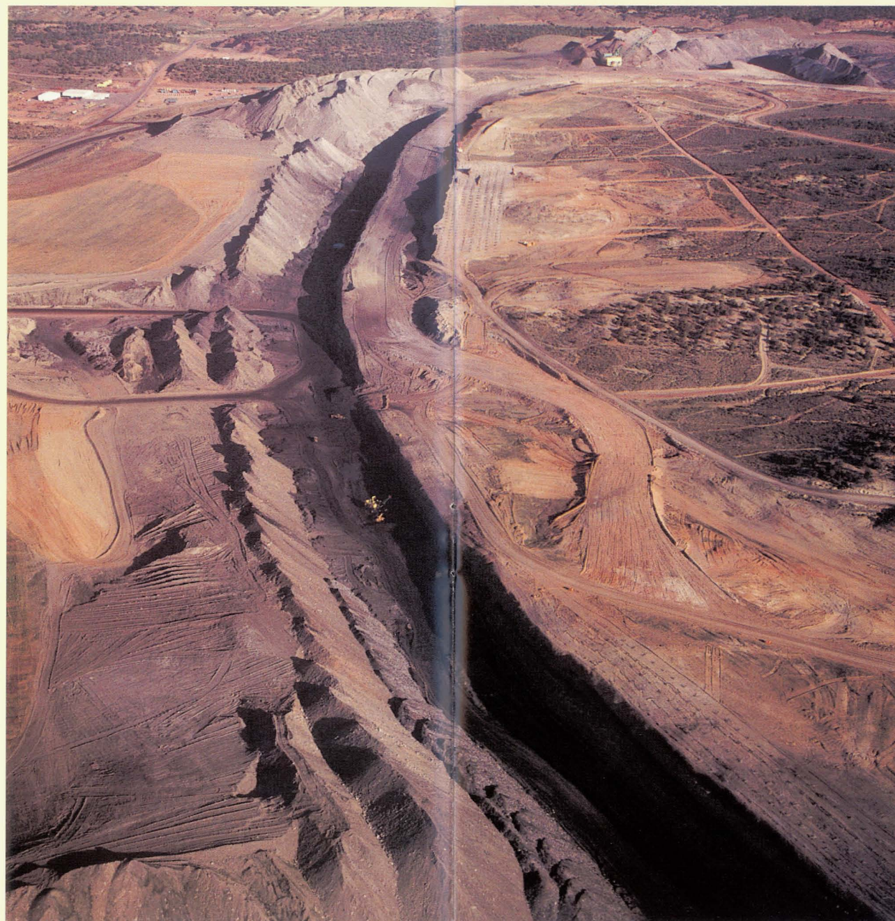
Coal lies up to 180 feet below topsoil, shale and rock. Once this material is removed, the coal is loaded onto trucks from the pit, which may stretch for 4 miles and be 80 to 150 feet wide.
