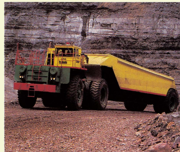
Haul trucks carry up to 300 tons of coal per load from active mining pits to hoppers for crushing and weighing.
