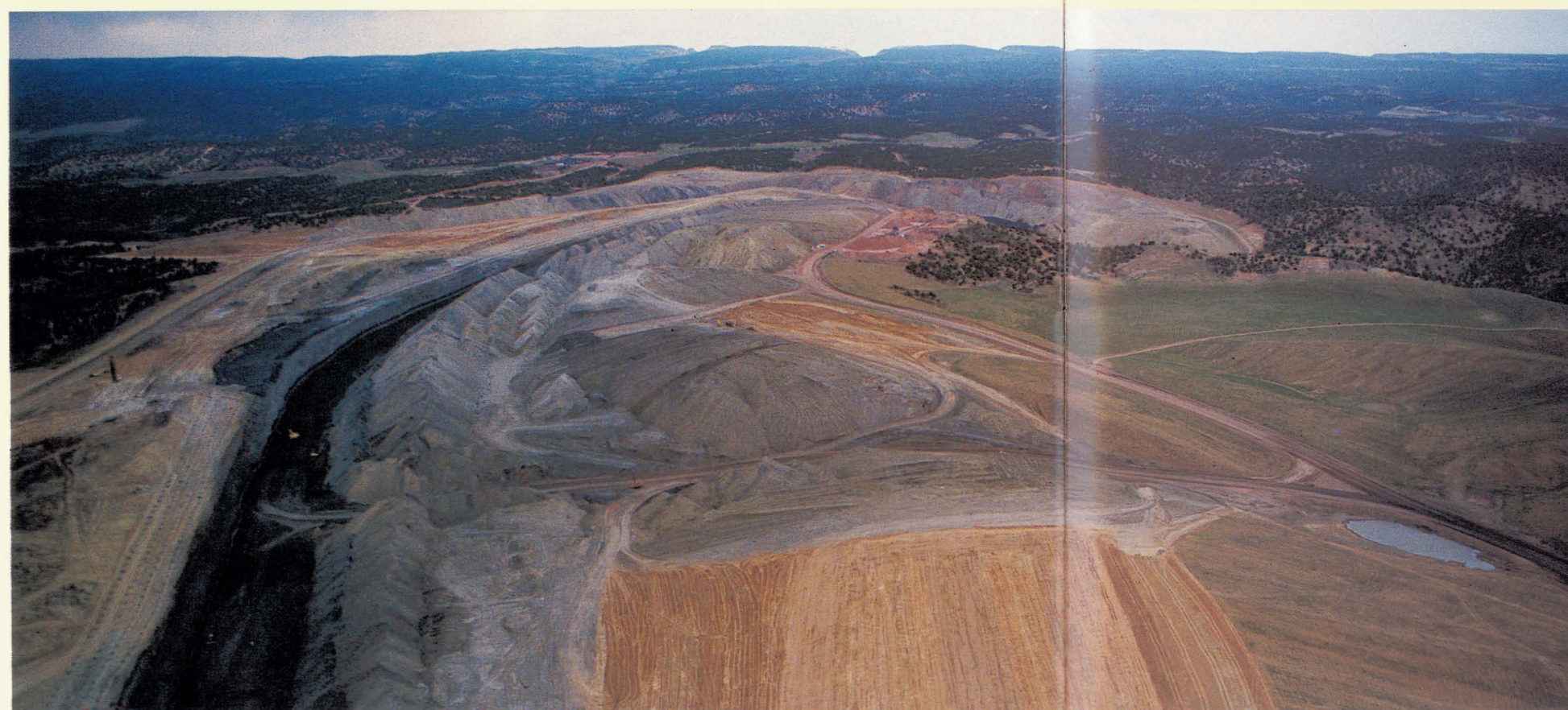
The mining and reclamation sequence as it proceeds from left to right: A) topsoil removal, B) drilled highwall, C) active pit, D) spoil piles, E) grading of spoil, F) topsoil replaced and G) revegetated land.
